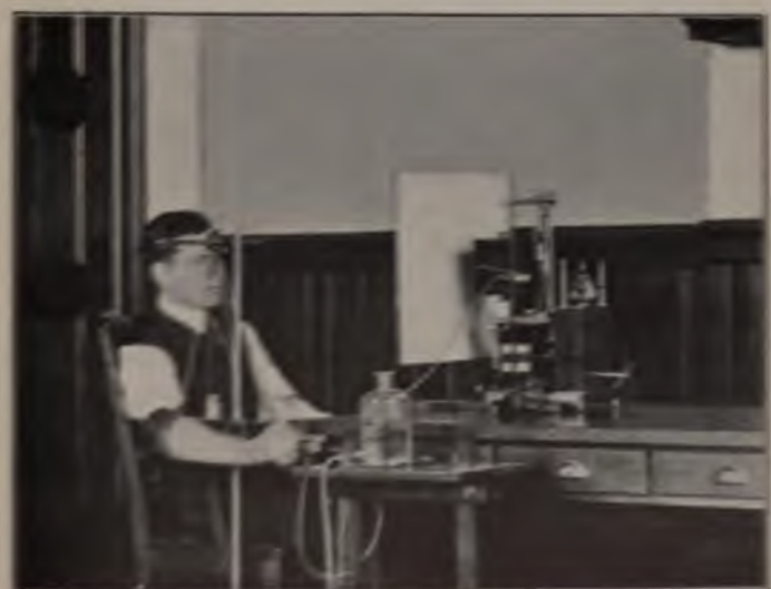
FIG. 56.—Plethysmograph. For recording changes in the volume of the arm, that accompany changes in the mental state.
